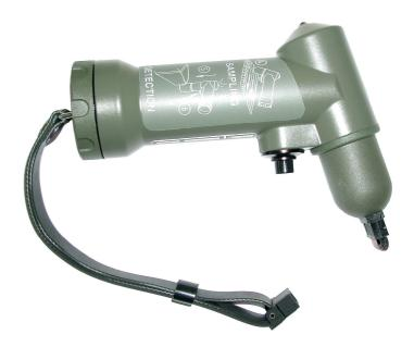
The S4PE is used with the AP2C and AP4C to detect very persistent agents in a liquid or frozen form. For example, Vx does not give any vapor at ambient temperatures. It is therefore impossible to detect Vx with a standard gas detector.
